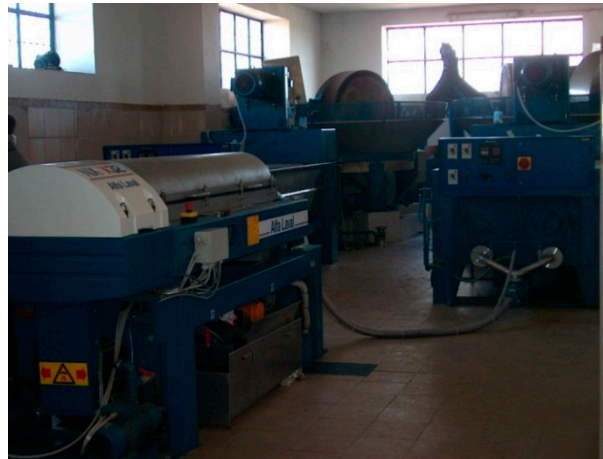
Figure 2. Machines that are pertinent to different working cycles side by side in the tested olive oil mill: the roller crusher (traditional discontinuous working cycle) and the decanter (modern continuous working cycle).
