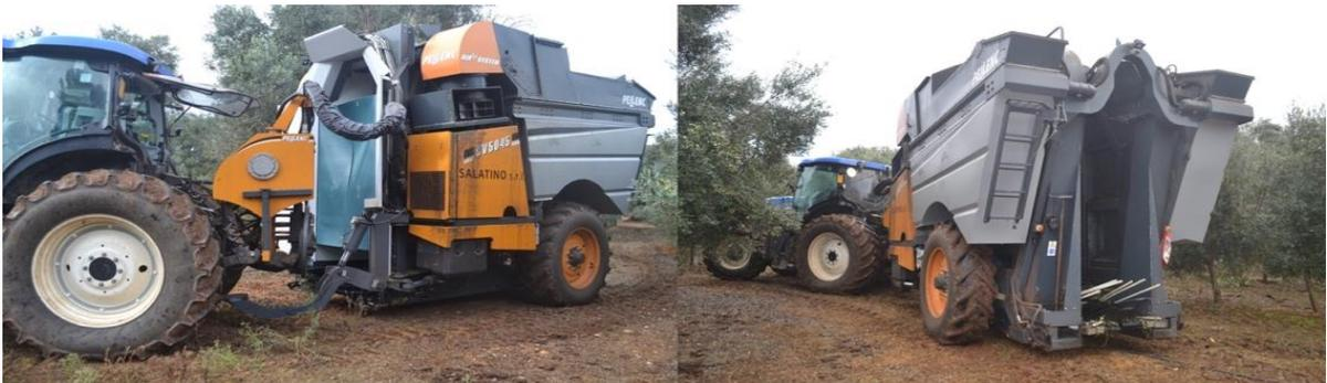
Figure 1. Towed olive harvester CV5045 built by Pellenc
