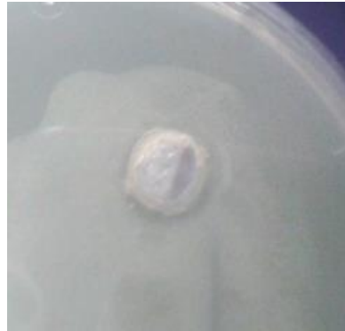
Ti coated with C_2H_4/H_2O
