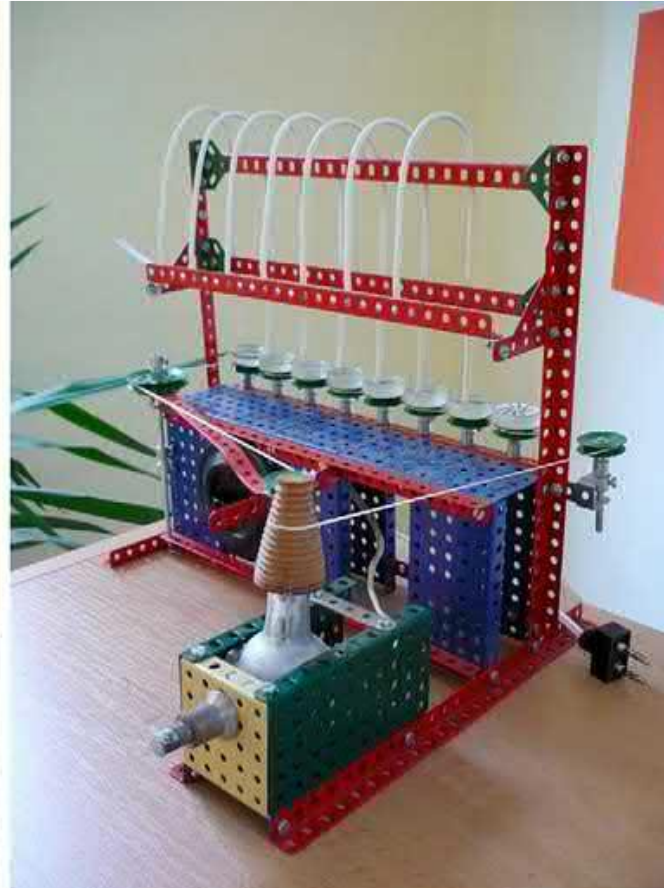
Otto Wichterle (1913–98) and he centrifugal casting apparatus he used to create the first soft, hydrogel contact lenses. (Photo by Jan Suchy, Wikipedia)
