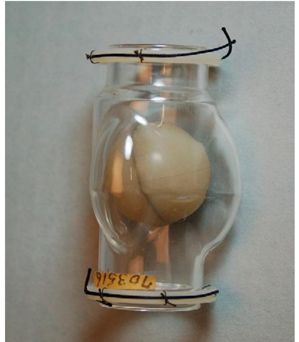
The Hufnagel heart valve, consisting of a PMMA tube and nylon ball
