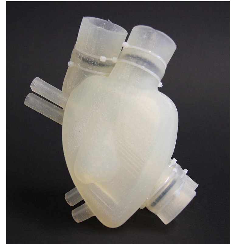
Soft Total Artificial Heart, ETH Zürich work in progress, 2019
