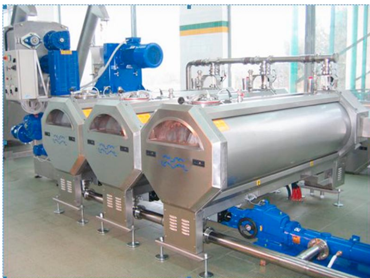
FIGURE 9.2 An innovative malaxer in a industrial plant. This new machine has been used in experimental tests carried out during the 2007/08 season in order to study its effect on the healthy and organoleptic properties of olive oil.
