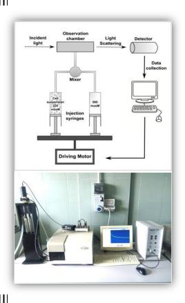
Stopped-flow light scattering (SFLS) is among the most widely used biophysical methodologies to assess the membrane permeability to neutral solutes and water of whole cells, organelles, sealed membrane vesicles as well as artificial liposomes. Membrane solute and water permeability are assessed by measuring the changes in light intensity scattered by the specimen shrinkage or swelling following osmotic or chemical gradients opportunely created across the membrane specimen.
