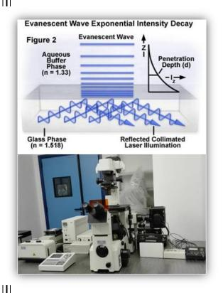
TIRFM is a well-established method to study water and solute permeabilities and cell volume regulation in cells of arbitrary shape and size. Adherent cells labeled with an aqueous-phase dye, are rapidly exposed to an osmotic gradient and the time course of fluorescence signal is detected.
