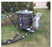
Figure 2.4: on the left: micro-ventilation system; on the right: thermal response test machine
