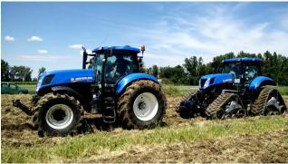
Figure 2.1: Wheeled and tracked version of the New Holland T7.260 during the test
