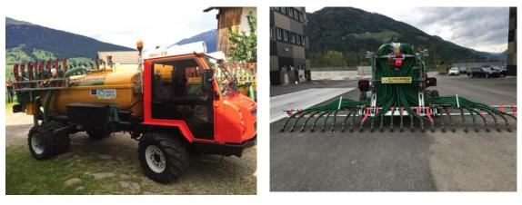
b Fig. 3.1: the self-propelled high-precision digestate spreader (a) and the low-emission spreading system
