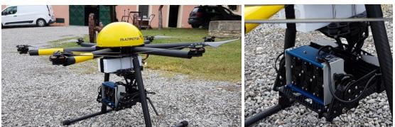
Figure 2 - Multirotor G4 Surveying-Robot (Service Drone GmbH) equipped with Tetracam MicroMCA multispectral camera (left); camera mounted on UAV gimble and ready to capture images (right).
