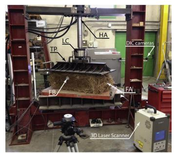
Figure 2.1: The test apparatus. HA is a hydraulic actuator; LC is the load cell; TP is a customdesigned top plate. The laser scanner has been placed so that the entire face FA and half of face FB could be acquired.
