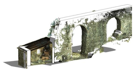
Figure 3.2: Historic Building Information Modeling (HBIM) built by point-cloud.
