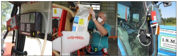
*Figure 2.3: Sampling of the operator exposure with personal samplers placed: (1) inside the tractor cab; (2) on the operator; (3) on the tractor, close to the cab door.*
