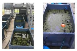
*Figure1: The pilot plant for Lemnaceae growth on diluted wastewater. On the left a general view is showed, on the right a particular of a tank with growing Lemnaceae fronds.*
