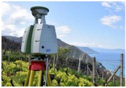
Figure 2.2: (a) Agricultural terraces of Costa Viola; (b) The Terrestrial Laser Scanner used.
