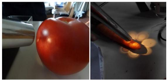
Figure 2.1: Particular of the spectral acquisitions on tomato and carrot
