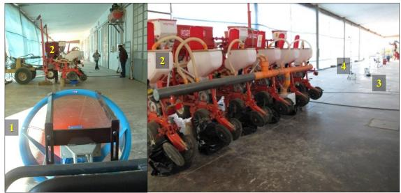
*Figure 2.1: Arrangement of sampling in the wind tunnel. (1) Fan generating the air flow. (2) Tested drill. (3) Sampling area with Petri dishes and (4) air pump samplers.*
