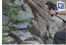
Figure 2.3: (a) Collapsed dry-stone retaining wall; (b) Use of DPI-8 to detect wall deformation.
