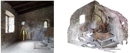
Figure 2.1: (a) Survey by Terrestrial Laser Scanner; (b)Mesh obtained by point-cloud extracted by photo of Digital Camera using software for Structure from Motion.
